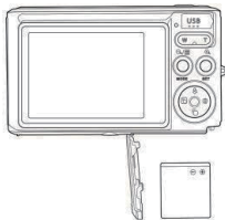
Install lithium battery
